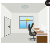
The sensor switches off the light whenever natural light exceeds pre-set daylight threshold, even no motion detected. with presence.
