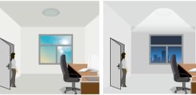
With sufficient natural light, the light does not switch on when presence is detected.
